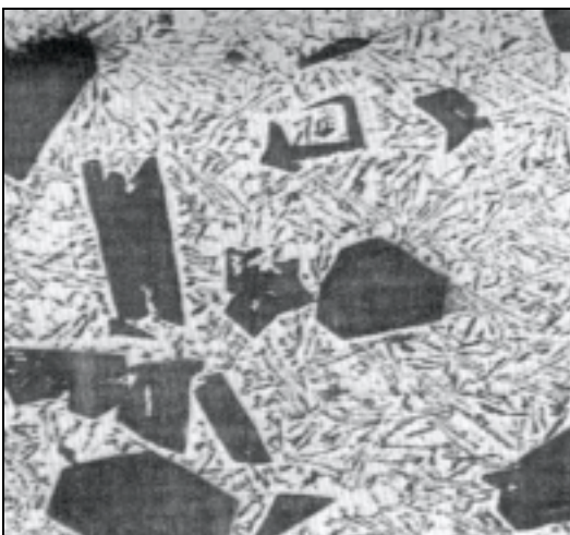
Fig. 1-9: hypereutectic alloy without phosphorus, SEM-magnification \Delta 100, [27].
