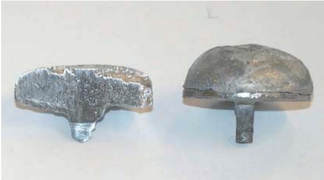
Fig. 7-6: Comparison of the remaining aluminium/cathode material after the experiment. To the right: aluminium and stainless steel; to the left: aluminium-copper alloy.
