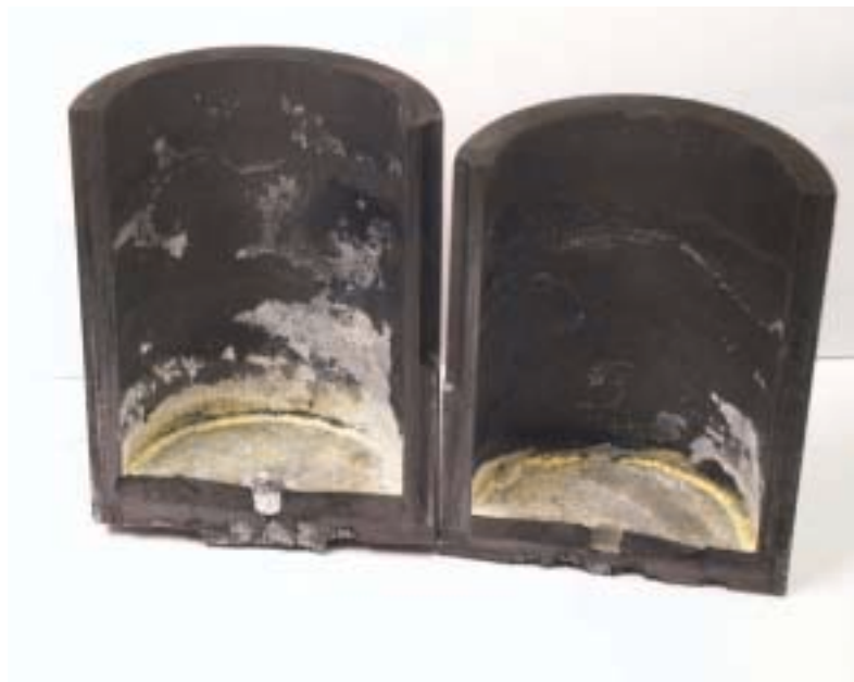
Fig. K-2: Cross section of empty crucibles after an experiment, showing the formation of Al_4C_3 (yellow colour) at the graphite bottom and partly on the side-walls (cathode material: copper).
