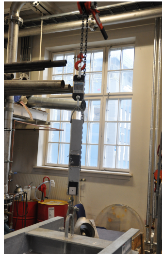
(b) Using a crane weight to measure the load
