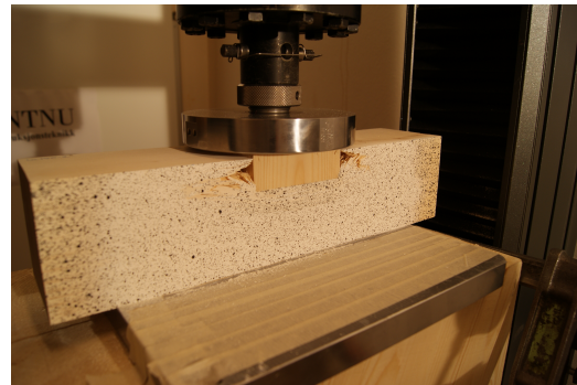
Figure 6.22: Local fracture mechanism
