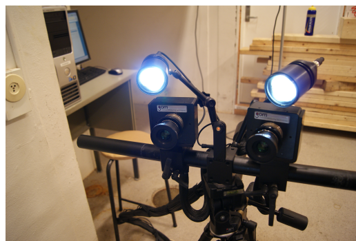
Figure 5.3: Cameras and light sources used for optical analysis
