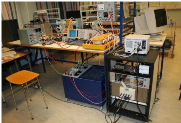
Figure 12.39: Photo of the experimental setup. To the left is the computer with the reference generator and the PWM. The LC-filter is placed on the table close to the computer, and the DC source is partly hidden by an oscilloscope. The step up transformer is placed on the left part of the table, and the load resistance is placed on the floor below the table. The rack contains measurement equipment and a power converter, and a computer with the FPGA board included is placed on the top of the rack.
