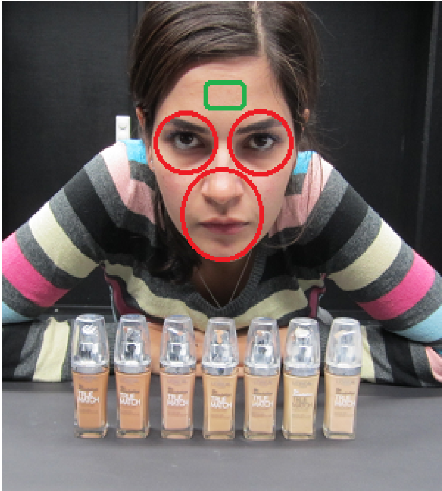
Figure 21: The Red circles indicate the areas in shadows or illuminated, the green square shows a potentially good area that can be selected for further processing. We carefully selected the appropriate areas based on the illumination trying to find the areas that have gained similar amount of light to the bottom of the foundation bottles that were least curved and thus glossy.
