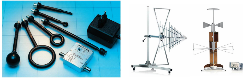
Figure 2.11: Rohde & Schwarz probe set for E and H near field emission (left). Rohde & Schwarz far field antennas, HL 561 and AM 524 (right). Pictures reproduced with permission from Rohde & Schwarz.
