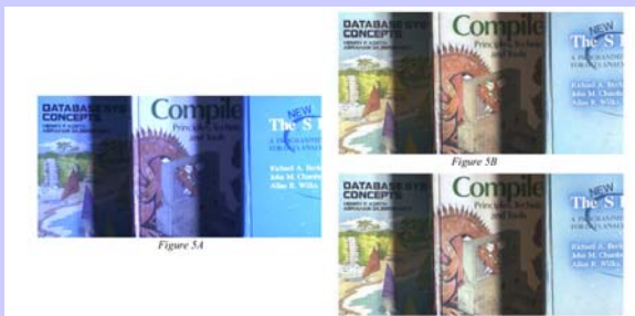
Figure 5: A: Input with blue color cast created by scene illumination for which the camera was not balanced. The image also has extended dynamic range obtained by frame averaging. B: Output from the McCann99 4-iteration. C: Output from the Franklin-McCann 4-iteration. The results here can be compared with those of Barnard [1]. Note that both the input and output images have been adjusted with postcuts for printing. The actual retinex input image is in log space.
