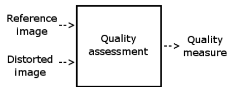
Figure 1: Full-reference image quality assessment, where an original is available in the quality calculation. The final quality measure is based on information extracted from both the original image and the distorted image.
