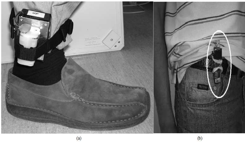
Figure 9: Attachment of the sensors (a) ankle (b)hip [69, 70].
