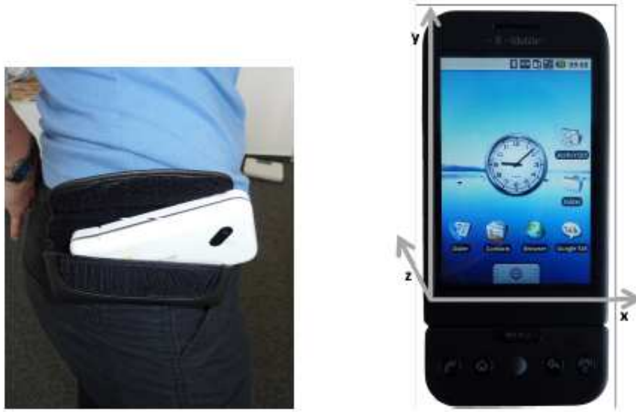
Figure 10: Mobile phone attachment to subject's hip to measure acceleration in 3D [73].
