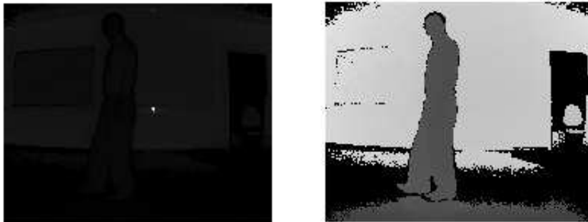
Figure 14: Example of ToF camera image: (a) intensity image (b) range image.
