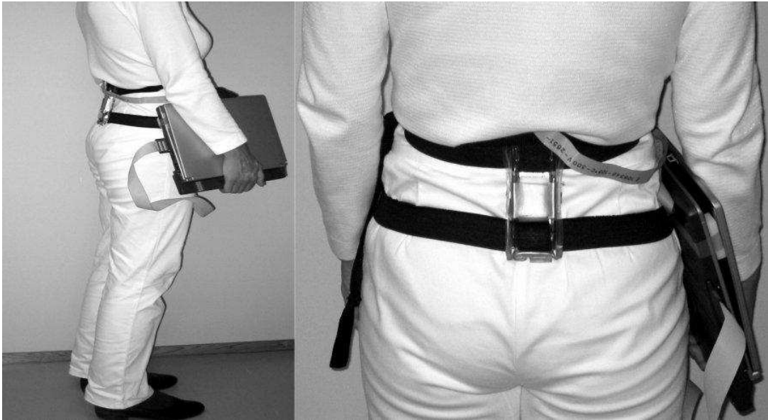
Figure 8: The experimental system for gait acceleration data collection [68].
