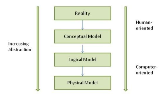
Figure 1: Levels of abstraction relevant to GIS data models. [4]
