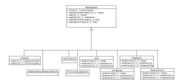
Figure 3: Road Segment UML model. [6]
