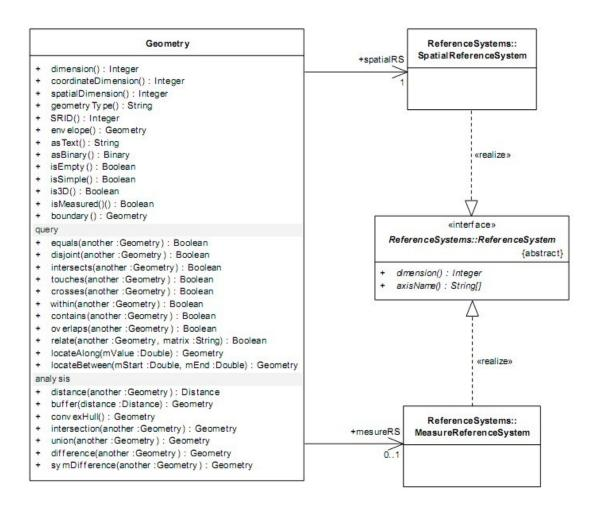
Figure 7: Geometry class operations [8]
