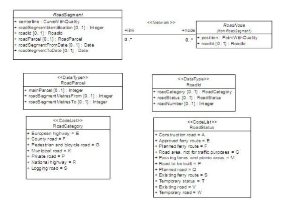
Figure 2: Road Network UML model. [6]
