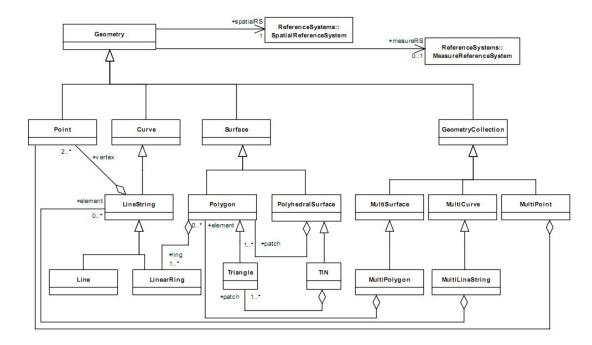
Figure 6: Geometry class hierarchy [8]
