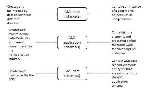
Figure 10: GML instance, application schema, and core schema. [16]
