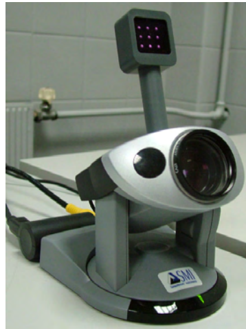
Figure 4: SMI remote eye tracker with infrared lightsource on top.
