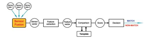
Figure 36: Fusion at sensor level [7].
