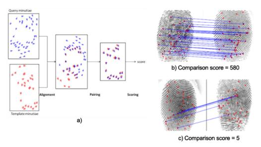
Figure 21: Fingerprint comparison by VeriFinger SDK 6.5. a) Flow diagram of a minutiae-based comparison algorithm. b) A genuine comparison of fingerprints with 30 matched minutiae, and c) an imposter comparison with 5 matched minutiae. Matched minutiae are connnected by blue lines. The comparison score (is calculated based on matched minutiae and some other functions that are defined by Neurotechnology.
