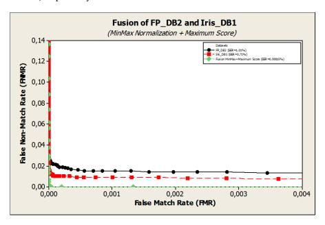
Figure 73: Scenario 3: Multi-modal Performance of Iris and Fingerprint using TanH Score Normalization + Simple Sum Score Fusion.  $EER_{FP\_DB2} = 1.01\%$ ,  $EER_{Iris\_DB1} = 0.71\%$ ,  $EER_{Finger+Iris} = 0.00015\%$ .
