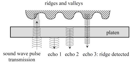
Figure 12: Ultrasound sensor (basic principle) [1].
