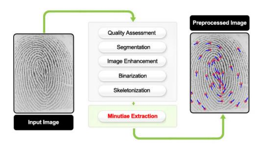
Figure 20: Flow diagram of the minutia-based pre-processing technique.
