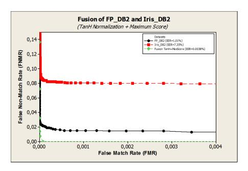
Figure 74: **Scenario 4:** Multi-modal Performance of Iris and Fingerprint using TanH Score Normalization + Simple Sum Score Fusion.  $EER_{FP\ DB2}=1.01\%$ ,  $EER_{Iris\ DB2}=7.35\%$ ,  $EER_{Finger+Iris}=0.0038\%$ .
