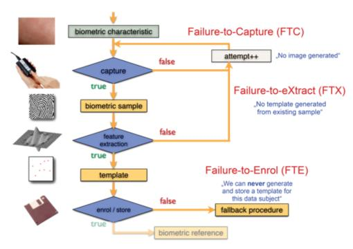
Figure 58: Potential failures in a biometric processing pipeline.
