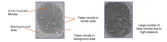
Figure 14: Poor image quality fingerprint image acquisition challenge [3].
