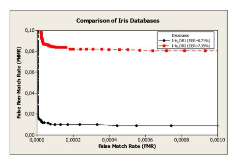
Figure 69: Comparison of Iris Databases.  $EER_{Iris\ DB1} = 0.71$  % and  $EER_{Iris\ DB2} = 7.35$ %.
