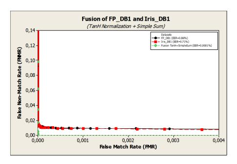
Figure 71: Scenario 1: Multi-modal Performance of Fingerprint and Iris using TanH Score Normalization + Simple Sum Score Fusion.  $EER_{FP\_DB1} = 0.86\%$ ,  $EER_{Iris\_DB1} = 0.71\%$ ,  $EER_{Finger+Iris} = 0.00010\%$ .
