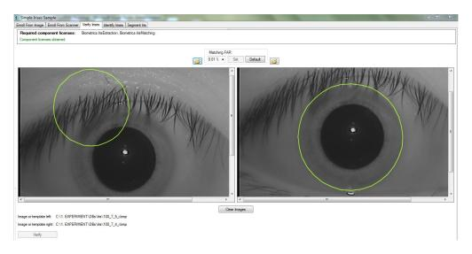
Figure 53: Iris image without segmentation. VeriEye has incorrectly segmented the iris (same iris comparison score=1.1120).
