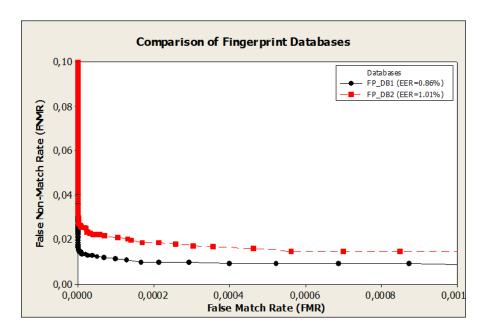
Figure 68: Comparison of Fingerprint Databases. EER<sub>FP DB1</sub> = 0.86 % and EER<sub>FP DB2</sub> = 1.01%.
