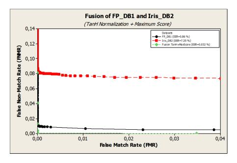
Figure 72: **Scenario 2:** Multi-modal Performance of Iris and Fingerprint using TanH Score Normalization + Maximum Score rule Fusion.  $EER_{FP\_DB1} = 0.86\%$ ,  $EER_{Iris\_DB2} = 7.35\%$ ,  $EER_{Finger+Iris} = 0.0320\%$ .
