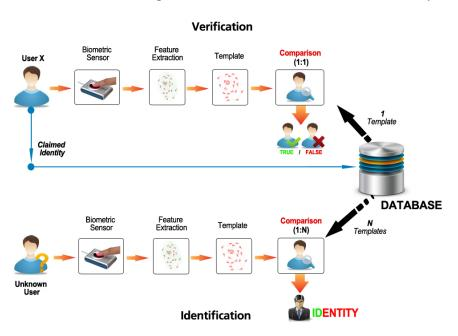
Figure 8: Schematic representation of the processing steps of a biometric system (verification and identification stage respectively).
