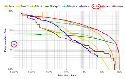
Figure 1: Detection Error Trade-off (DET): False Match rate (FMR) vs. False Non-Match Rate (FNMR) [22].
