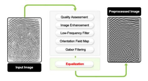
Figure 22: Flow diagram of the correlation-based pre-processing technique.
