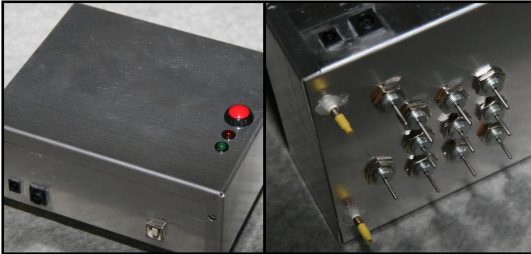
Figure 8: On the top we see one button and two status lights, the function of these are controlled by software. The inputs on the side of the box are 9V DC input, 12V DC input and a USB connector for programming. Underneath we see 11 pins that push the keys 0 to 9 + ENTER. The legs are adjustable and make it possible to use on different keyboards.
