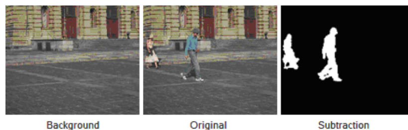
Figure 6: Background segmentation for extracting the silhouette picture (subtraction)[13].
