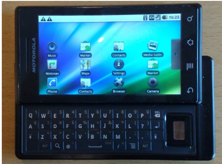
Figure 13: Motorola milestone, a smartphone with a builtin triaxial accelerometer.
