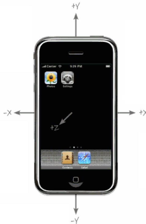
Figure 2: Description of the orientation of the accelerometer in the iPhone. Illustration from [6].
