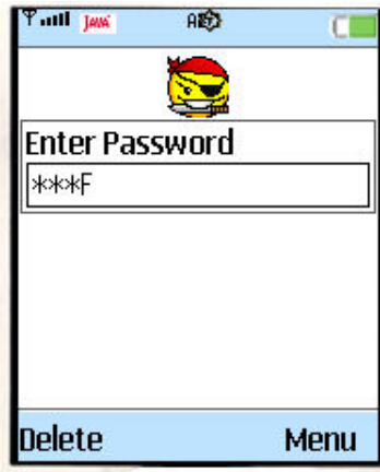
Figure 21: The last entered character must be visible, because many different letters maps to the same button.
