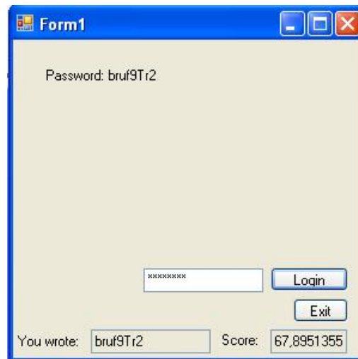
Figure 5: This program returns a score. It is similar to imitation program one, but it returns the score instead of an “Accepted/Fail”. This means that attackers will get a little more information about how their typing is compared with the victim’s typing.
