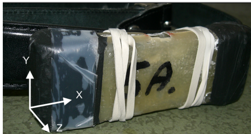
Figure 11: The MR100 sensor, with the three directions noted.
