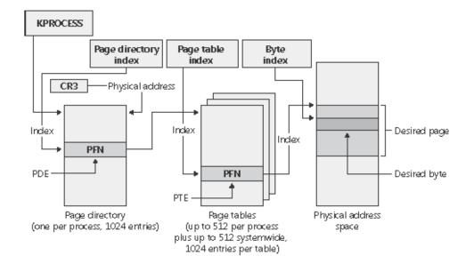
Figure 7: Virtual to physical address translation process [88]
