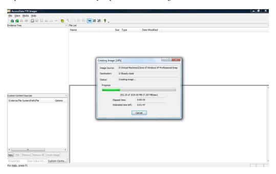
Figure 9: Imaging process of physical Memory by FTK Imager
