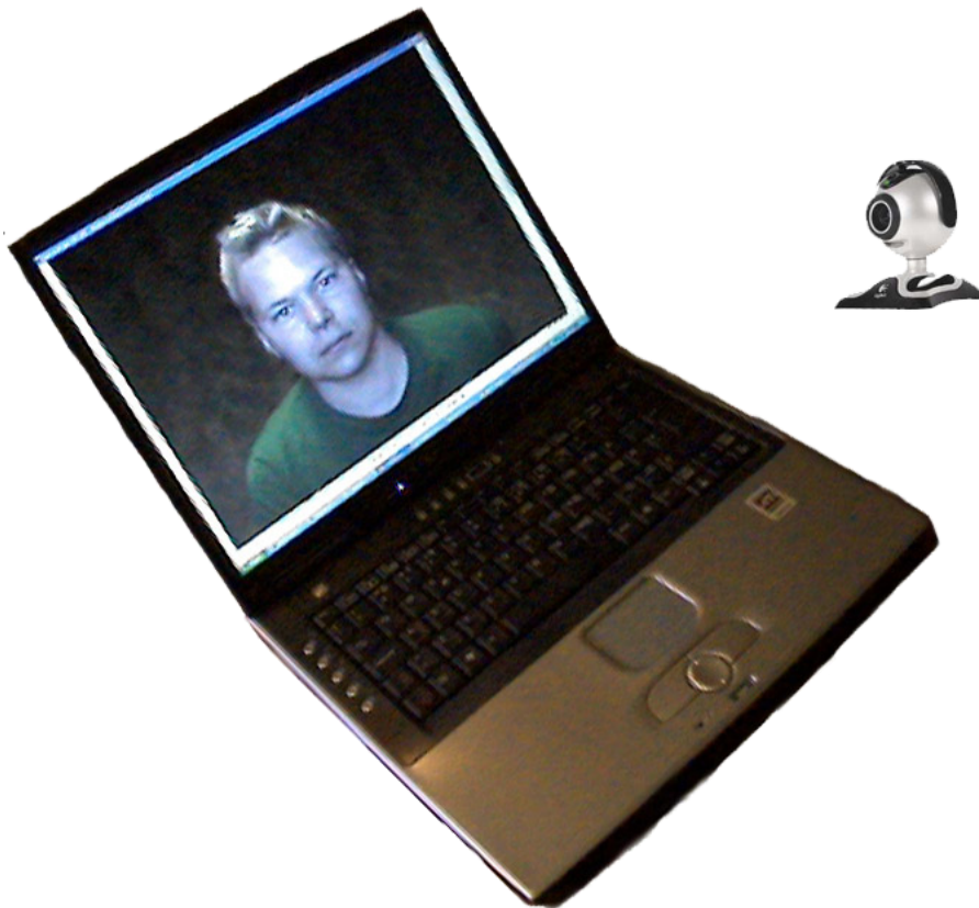
Figure 4: This illustrates how the PC may be placed in front of the web-camera, attempting to fool the face recognition based authentication mechanism.
