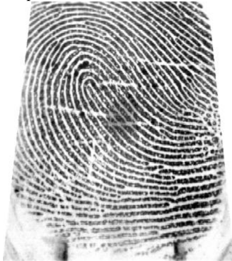
Figure 6: A fingerprint image with minutiae details and sweat pores visible. Fingerprint captured with a digitalpersona U.are.U® 4000 Sensor [Digi] and Verifinger Demo Software [Neur].
