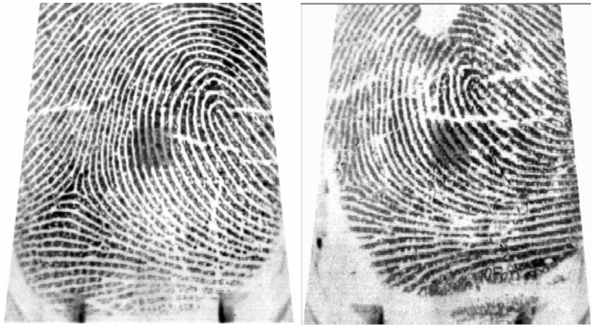
Figure 12: Images captured from the experiment. Fingerprint of a real finger, to the left, and fingerprint of the artificial finger, to the right.
