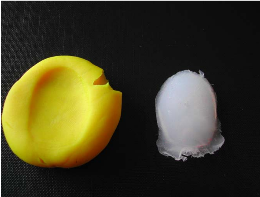
Figure 14: Fingerprint mould in a lump of clay and an artificial fingerprint made of Silicone.
