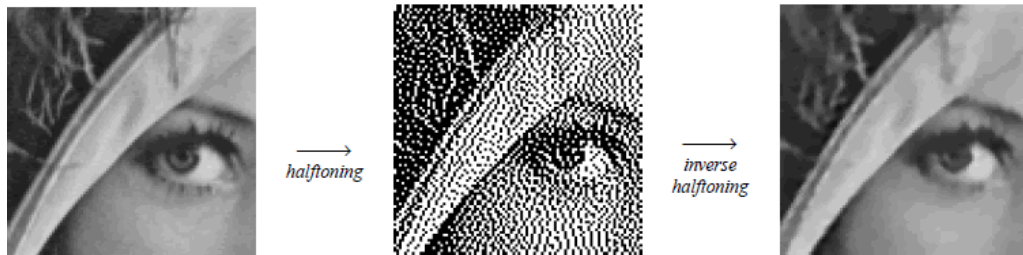
Figure 2: An illustration of halftoning and inverse halftoning. Detail of the Lena image: original (left), Jarvis error diffusion halftone (centre), and inverse halftone result (right). From Foi et al. [6]
