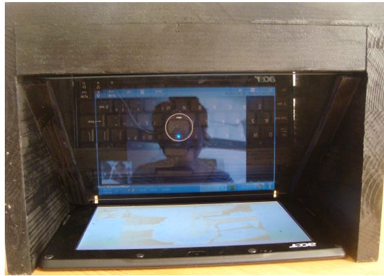
Figure 16: The hardware solution teleprompter model. The display laid flat, its reflection shown in the glass. The camera placed at the location of the remote user's eyes in the image. The black wooden casing keeps out other illuminations, preventing the desired reflection from being disturbed.
