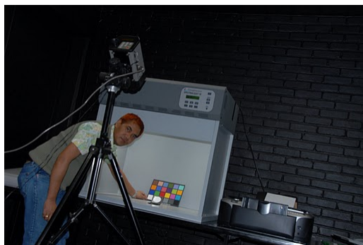
Figure 64: Setup for measurement of SPD
