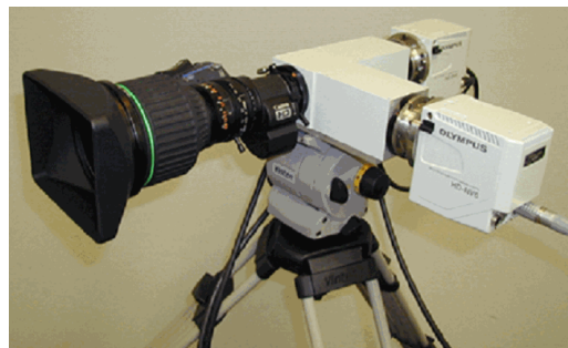
Figure 26: 6-band HDTV camera [Source: Ohsawa et al. (2004)]
