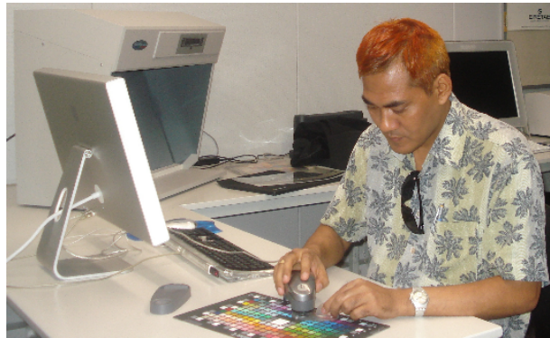
Figure 66: Measuring spectral reflectances
