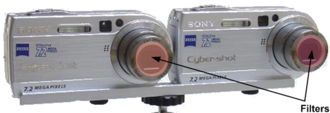
Figure 27: Illustration of a multispectral-stereo system with two cameras and two filters
