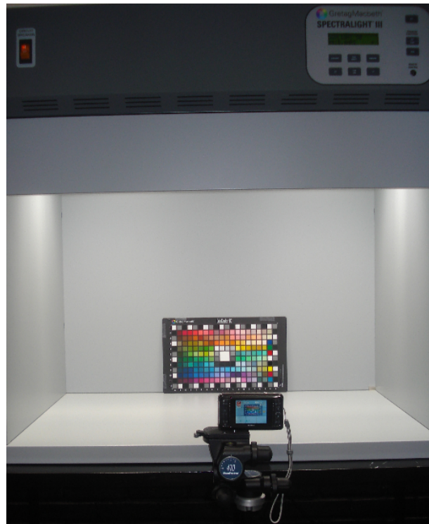
Figure 67: Multispectral image capture of a Macbeth color checker
