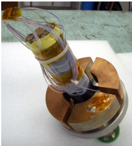
Fig.4.18. Cable inside model connected to heat exchanger
