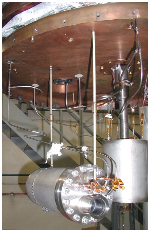
Fig.4.22. The model during the connecting to the cryostat
