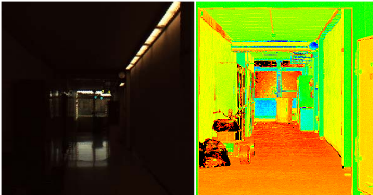
Figure 22. Image and point cloud got from Leica HDS3000 .
