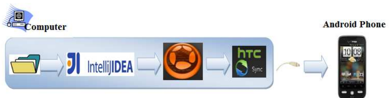
Figure 5: Shows the flow process from computer. On the computer we have our project folder, which is created and edited by the development team in IntelliJ IDEA. Building the project is done in Corona Simulator, which outputs an .APK file. HTC sync is also installed on the computer and can transfer this file to the android device.
