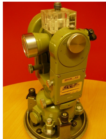
Fig 1. An 'old-fashioned' theodolite fitted with a spacer
