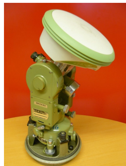
Fig 2. GNSS antenna mounted directly on the telescope
