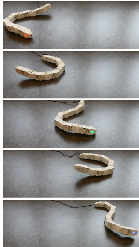
Fig. 4. Mamba sidewinding across the floor.
