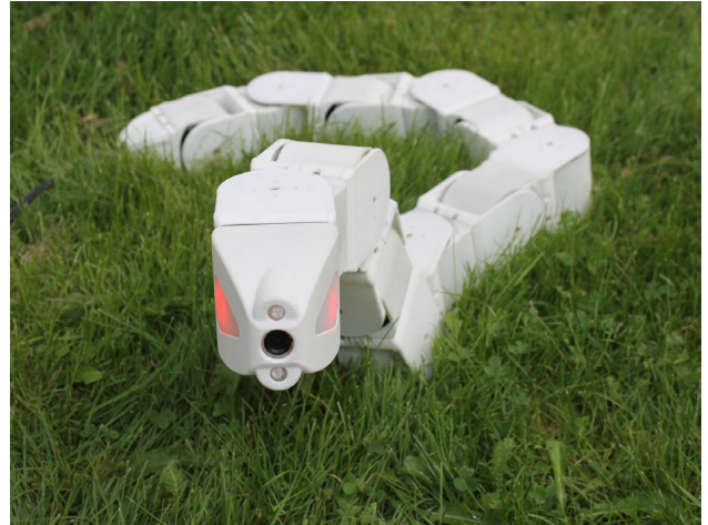
Fig. 1. The snake robot Mamba .
