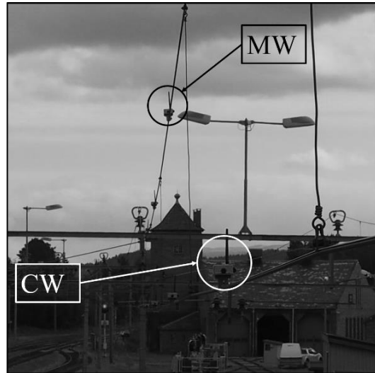
Figure 5: Field measurement set-up: sensors are mounted on contact (CW) and messenger wires (MW).
