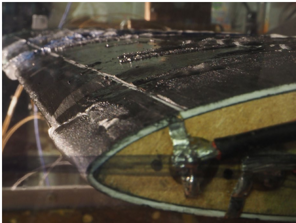
Figure 14. Anti-icing test. Partial ice accretion can be seen near the window and on the external thermocouples due to insufficient heating.
