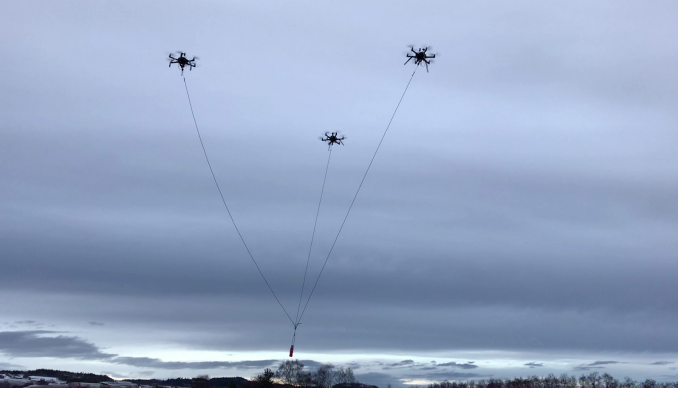
Fig. 1. Image of the experiment. From left to right, we see multirotors 1, 3 and 2. The wind was blowing heavily from right to the left, so it is apparent that more force from the suspended load is applied to the rightmost multirotor.
