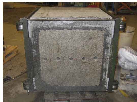
Fig. 4. The concrete-granite block for test in group 2.
