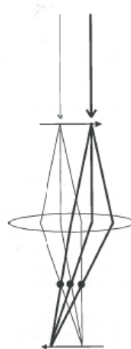
Figure 2.12: The pathway of the electron beam through the intermediate lens to the image plane. The beam is deflected stronger by the intermediate lens [45].
