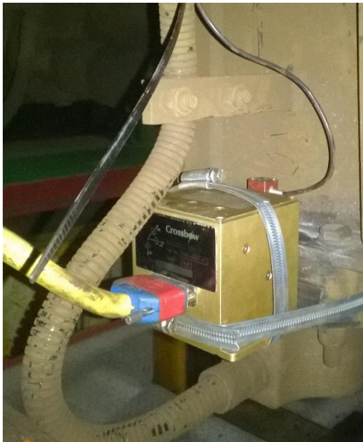
Figure 2. Bogie mounted gyrometer and accelerometer
