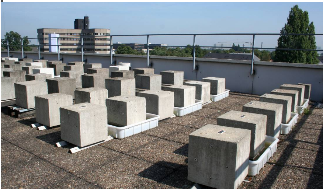
Figure 3: Concrete cubes located at the outdoor exposure site in Düsseldorf, Germany
