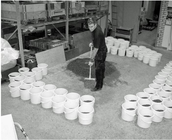
Figure 19: Fractional shovelling, in accordance with EN 932-2.
