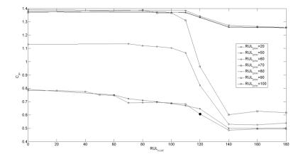
**Figure 8.** Average maintenance cost  $C_{av}$  vs threshold RUL<sub>rconf</sub> with  $C_d = 0, C_i = 30, C_p = 80, C_c = 100.$
