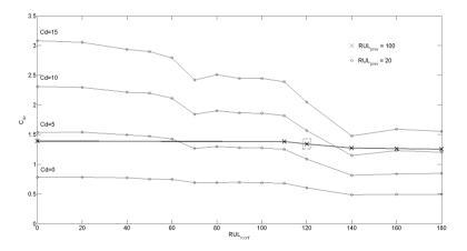
**Figure 9.** Impact of unavailability cost  $C_d$  on average maintenance cost vs threshold RUL<sub>rconf</sub> for RUL<sub>prev</sub> = 20 and 100.  $C_i = 30, C_p = 80, C_c = 100.$
