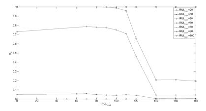
Figure 5. Average number of preventive replacements  $N_p$  vs threshold RUL<sub>rconf</sub>
