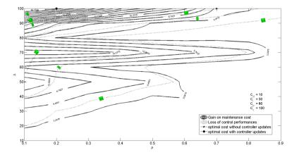
**Figure 12.** Bold (dotted) isolines delimit gain on maintenance cost (loss of control performances) areas provided by controller updates
