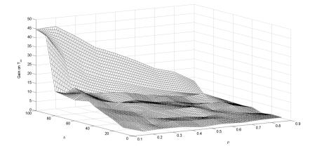
Figure 11. Gain on average renewal cycle  $T_{av}$  provided by controller updates
