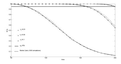
**Figure 2.** Reliability of the actuator when its degradation level  $d_i = 50$  is measured in phase 1 at  $t_i = 50$ .  $\alpha = 2, \beta = 1, a = 0.5, b = 0.75, L_1 = 100, L_2 = 300, L_f = 500$ .
