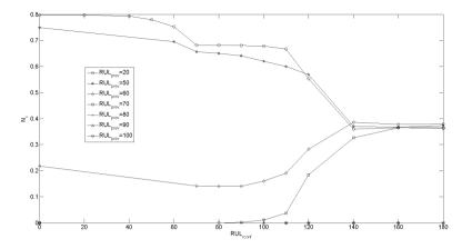
Figure 4. Average number of corrective replacements  $N_c$  vs threshold RUL<sub>rconf</sub>
