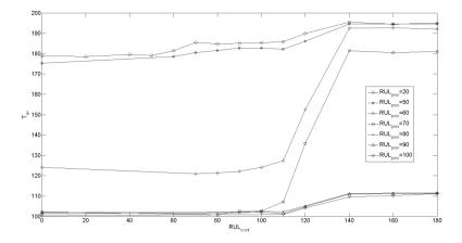
Figure 6. Average duration of a renewal cycle  $T_{av}$  vs threshold RUL<sub>rconf</sub>
