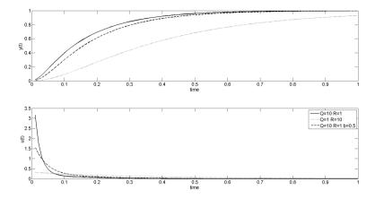
**Figure 1.** System output y(t) (up) and corresponding control input u(t) (down) for two LQR controller settings. The setpoint s(t) (not shown here) is a Heaviside step  $s(t) = 1 \forall t \ge 0$ .
