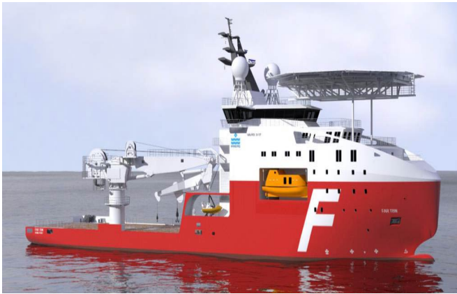
Fig. 1. Boomerang-shaped knuckle-boom crane on OSC vessel (courtesy Offshore Energy Today) [10].
