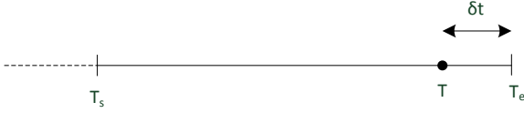
Fig. 3: The timescale of the real-time implementation. The thrust allocation algorithm is solved iteratively. The output signal is sent to the local thruster controllers at time T , and stays constant until time T_e when the output from the next iteration of the thrust allocation algorithm is available.
