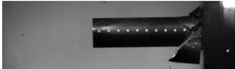
Figure 7: HRC 52 projectile impacting at 134.7 m/s captured by the high-speed video camera. Two shear fractures are evident.
