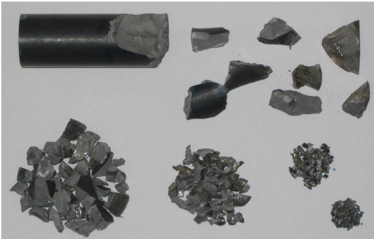
Figure 10: HRC 52 projectile after impact at 250.5 m/s. The fragments are sorted according to their size.
