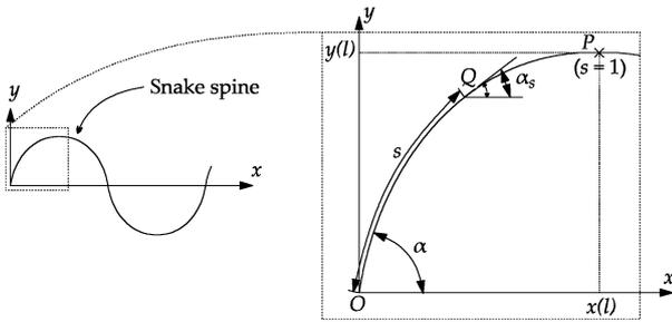
Fig. 5. The serpenoid curve.<sup>3</sup> By permission of Oxford University Press.
