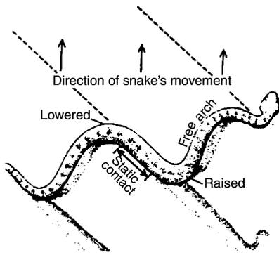
Fig. 3. Sidewinding locomotion<sup>26</sup> © 1993 IEEE.
