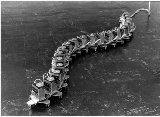
Fig. 1. The Active Cord Mechanism model ACM III.<sup>3</sup> By permission of Oxford University Press.
