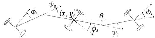
Fig. 4. The first three links of the ACM III employed by Ostrowski and Burdick.<sup>14</sup>
