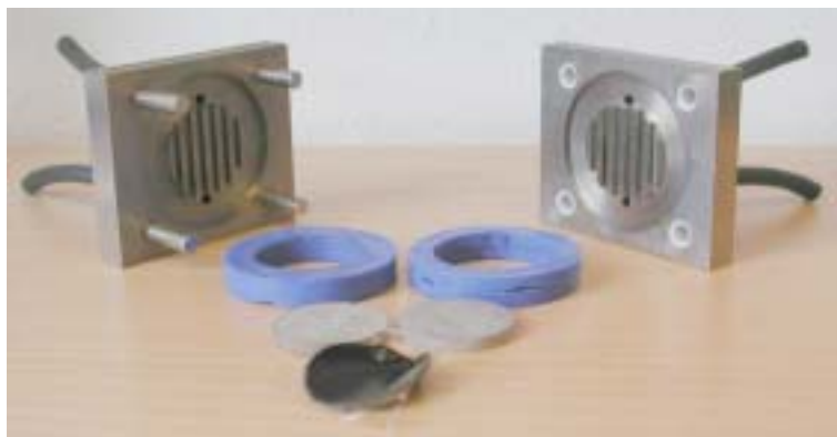
Figure 4.2: Picture of SPEcell together with fittings, Ti-sinters and one MEA.
