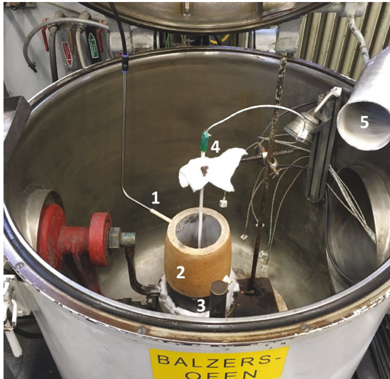
Figure 28. Furnace setup for remelting in molten heelwhere; 1=Argon gas inlet, 2=Hood, 3=Crucible, 4=Thermocouple and 5=Exhaust pipe. The temperature was measured by a thermocouple placed inside the melt, and the melt was flushed with argon introduced to the hood at 10 L/min. First, the crucible with approximately 1 kg of aluminium heel was heated to 780 °C. Then the furnace was turned-off to skim
