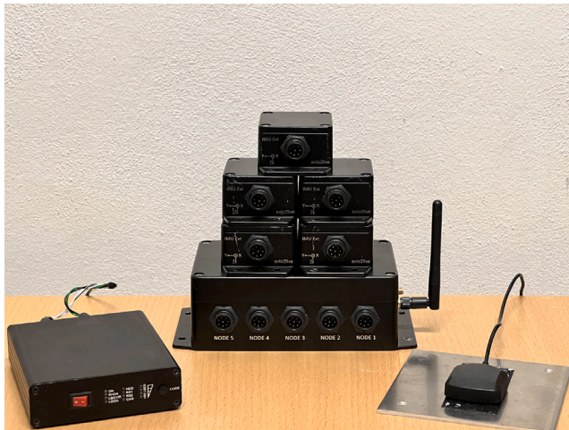
Fig. 12. Our data logging system comprises five IMUs, a GPS receiver, a solid state drive, and a synchronization unit.
