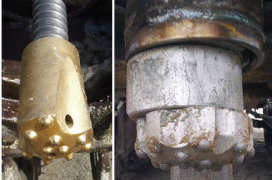
Figure 4. Left: Drill bit for self-drilling Ischebeck anchor (OD = 70 mm, 40 mm for the anchor rod). Right: Casing (OD = 139.7 mm) and eccentric drill bit (OD = 151 mm) for Odex 115 system.
