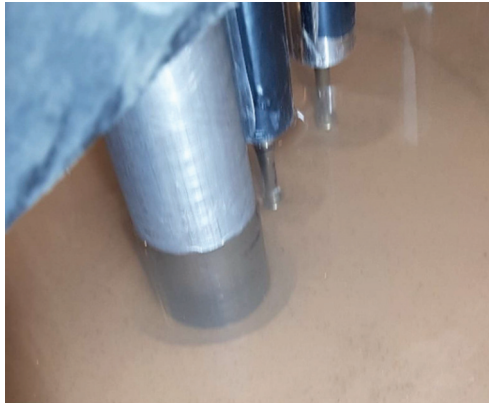
Figure 6-13. Local cavity at the soil surface around the pile casing after test W-4.
