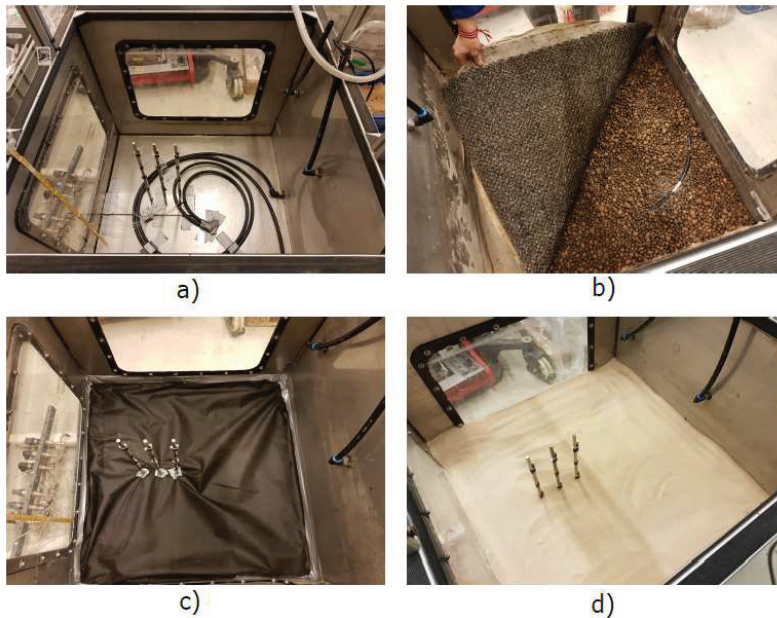
Figure 6-5. Stages in initial soil model preparation: a) support for pore pressure standpipes and perforated tubes for saturation and drainage of soil model; b) filter layer (LECA and geotextile); c) geotextile as separation layer; d) filling of dry sand.
