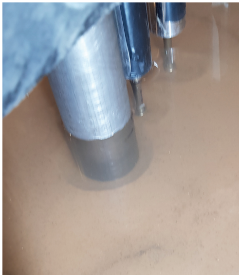
Fig. 12. Local cavity at soil surface around pile casing after test W-4. [Colour online.]
