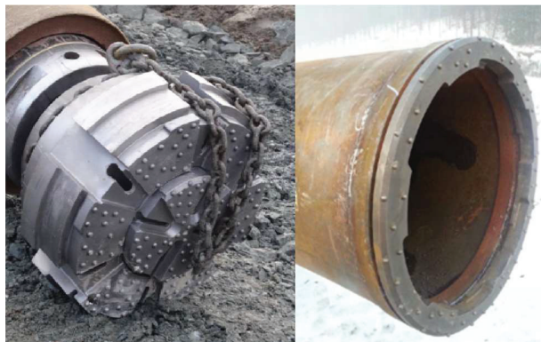
Figure 3-4. Concentric pilot- and ring bit system used to drill pile casings for the Skaudal Bridge. (Photo by Samson Degago and Ørjan Edvardsen, NPRA)
