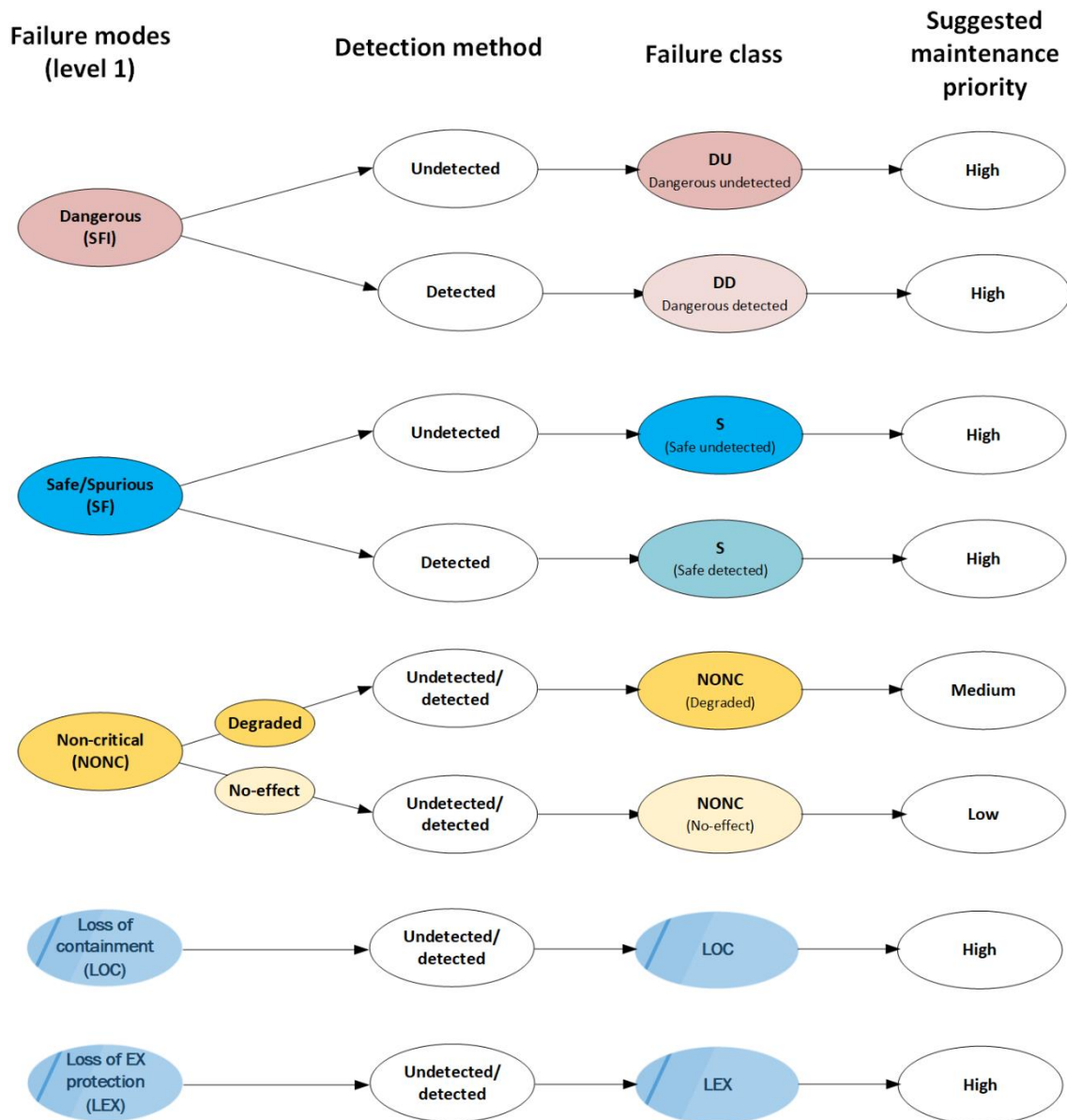
Figure 8: Automatic determination of failure class and maintenance priority (based on failure mode and detection method)
