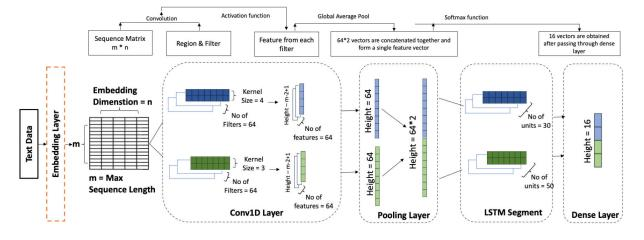
FIGURE 3. CNN-LSTM proposed model architecture diagram.
