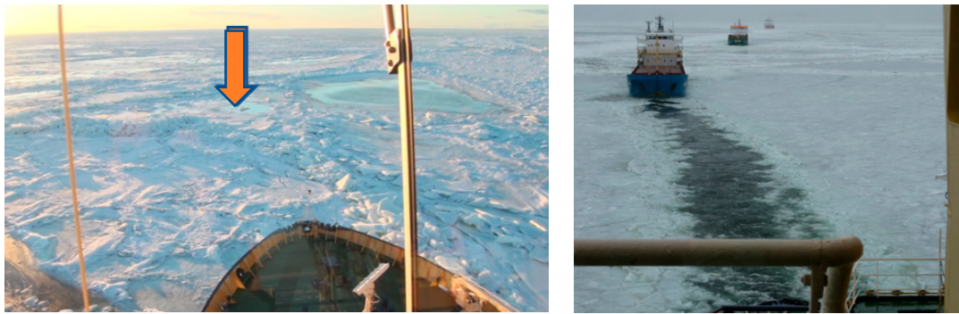
Figure 3. (Left) the icebreaker Frej, at 5 knots, is opening a new channel through the 30–55 cm thick ice. A minute after this photo is taken, by the red arrow, Frej is brought to a complete stop by this seemingly insignificant ice ridge that shows very little of its true size above the ice sheet. (Right) convoy service. Often the ships in the convoy become stuck and the icebreaker must go back and break them free. During this maneuver, the other ships become stuck. It is tedious work. Photo by the author.
