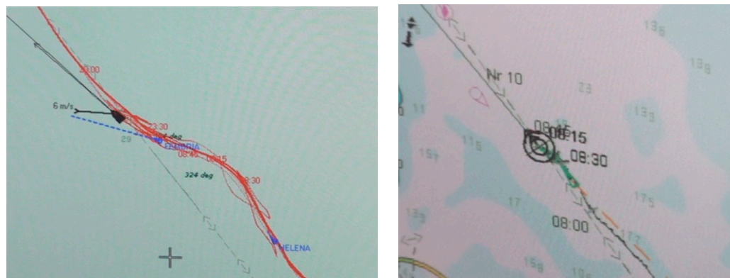
Figure 6. (Left) a screenshot from the Adveto ECDIS; the icebreaker is escorting a convoy of two ships at 8.45 in the morning. He is using the historic track of himself from about 23.00 the previous night, showing that the ice sheet has been relatively stable. To the (right) is a screenshot from the ship's regular Furuno ECDIS a little earlier. The historic track cannot be called up here. Photo by the author.
