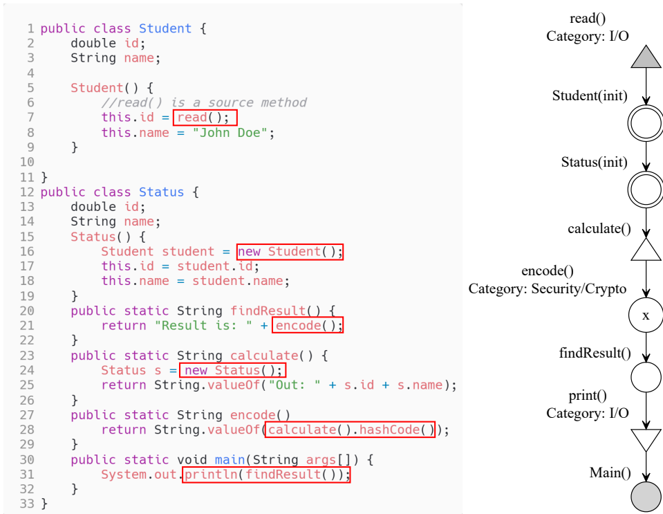
Fig. 1. Example of a privacy data-flow generated for a source code fragment and its abstraction
