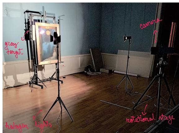
**Fig. 4** In-situ setup for hyperspectral imaging
